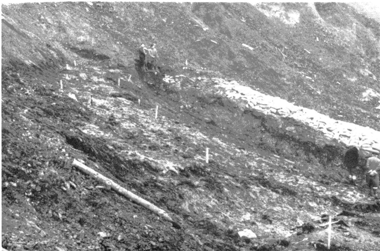
1.25* Colour transparency showing bowl in natural ground left by the slip. The pegs mark original ground surface.
