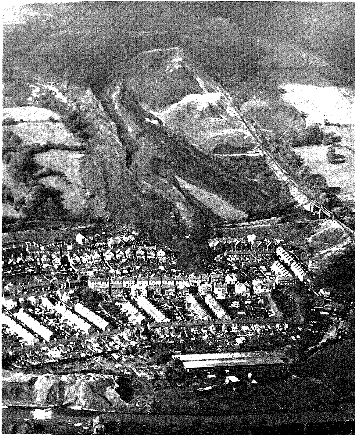
1.19 Photograph showing general view of flowslide and mud run. 21st October 1966, approx. 1 p.m.
